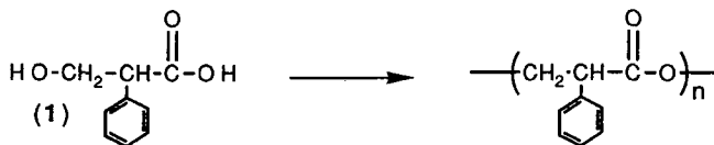
FIG. 1. Low temperature polycondensation of tropic acid.
